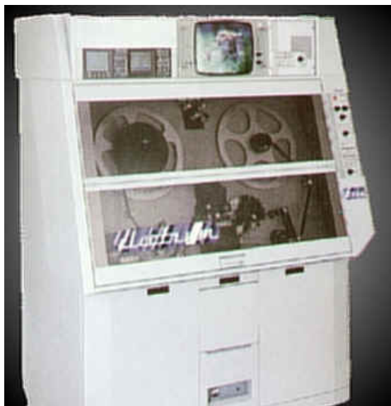
Flying spot scanner (CRT)
